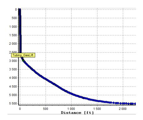
Fig. 3. The position of gas injection
