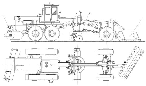
Fig. 2. Scheme of the proposed attachment mounted on the grader 1-a Front work tool with a rotary instrument; 2-a chain stroke work tool; 3-a brush
