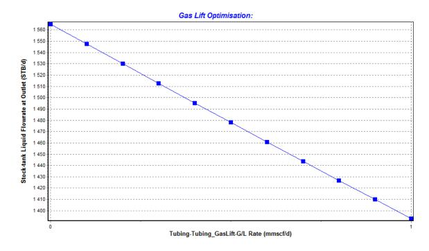
Fig. 1. Flowrate drop with increased gas-oil ratio in horizontal pipe
