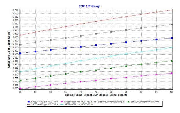
Fig. 6. The performance curve for ESP
