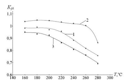
Fig. 1. Relative viscosity factor dependence on the test motor oil temperature
