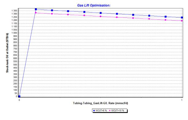
Fig. 4. The performance curve for Gas Lift
